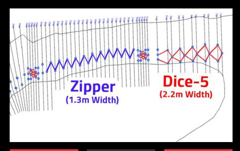
**REDUCED BLASTHOLE DEVIATION** (IMPROVED **ACCURACY**)
